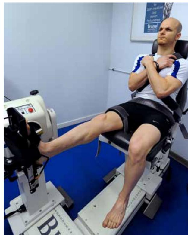
Above: Participant positioned for an ankle joint strength test on an isokinetic dynamometer
